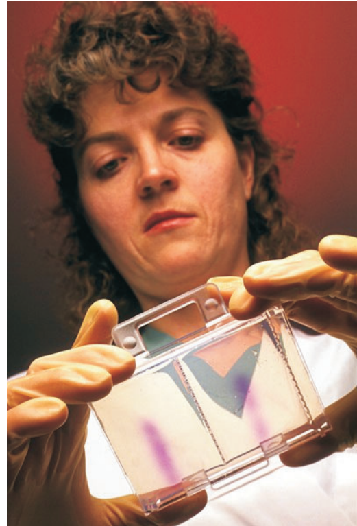
FIGURE 2. A dye is used to highlight the DNA segments as they pass through the gel in gel electrophoresis. (Courtesy, Agricultural Research Service, USDA)
