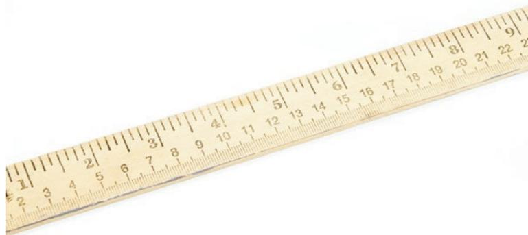
**FIGURE 2.** One side of this measuring stick is marked in inches and the other in centimeters.
